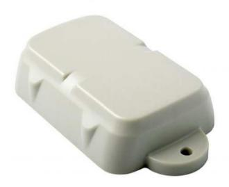
Rugged, waterproof, cellular GPS tracking device designed for tracking non-powered, exposed assets where super-long battery life is essential. The device works on 2G or 4G Cat-M1/NB-IoT networks and can be fitted with Lithium-Thionyl Chloride (LTC) batteries, for extended temperature tolerance. The innovative battery meter allows precise battery level monitoring and accurate battery life predictions.
